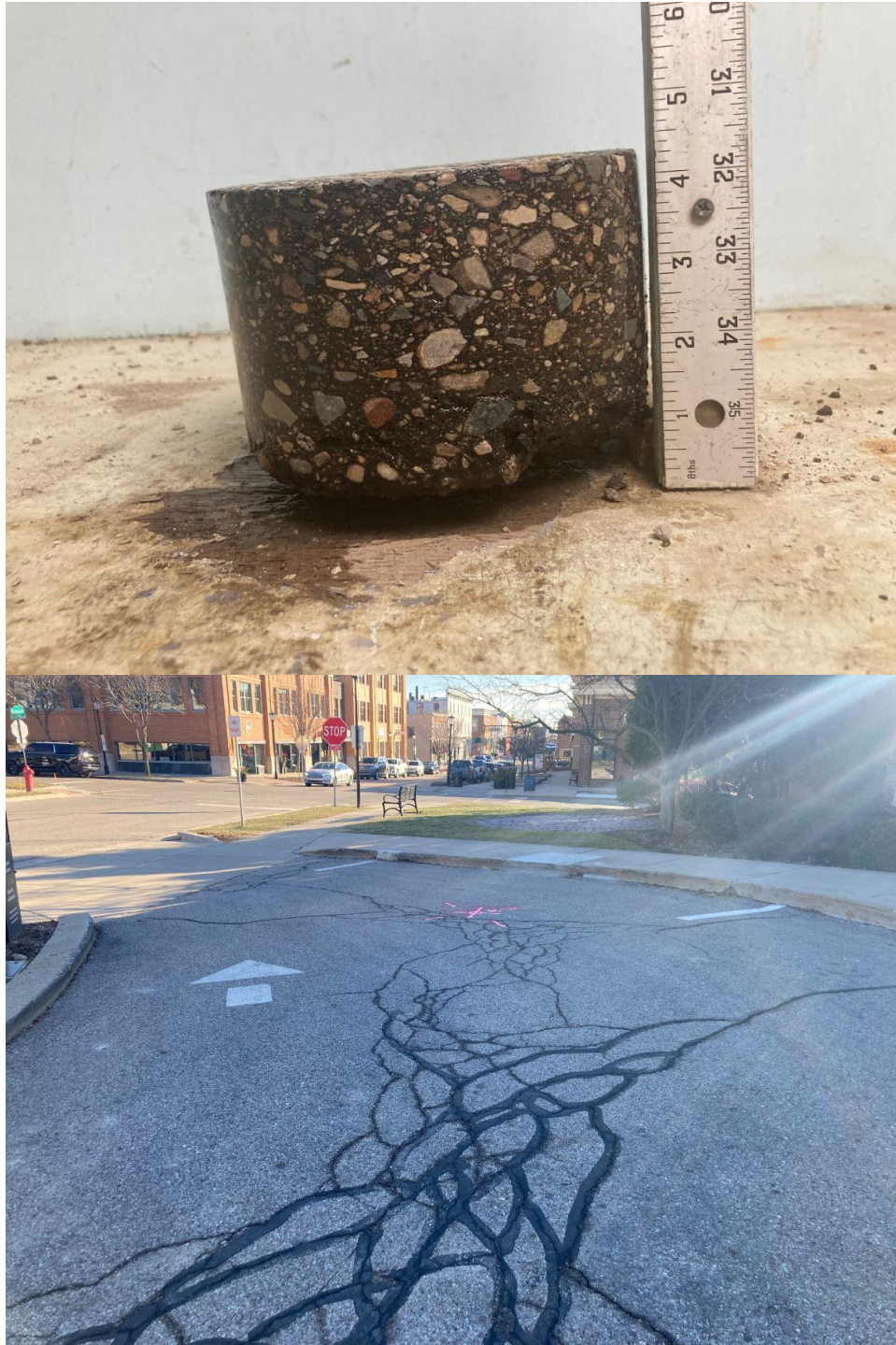
Core Photograph of B-6: Bituminous Concrete = 4-1/4 inches
