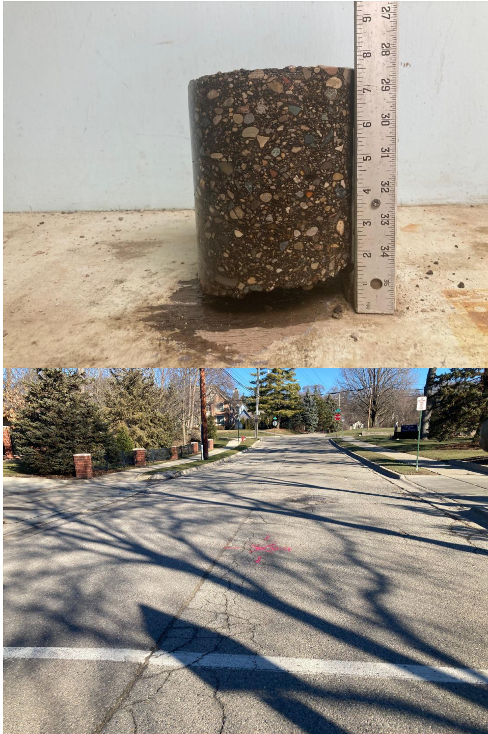
Core Photograph of B-4: Bituminous Concrete = 7-1/2 inches
