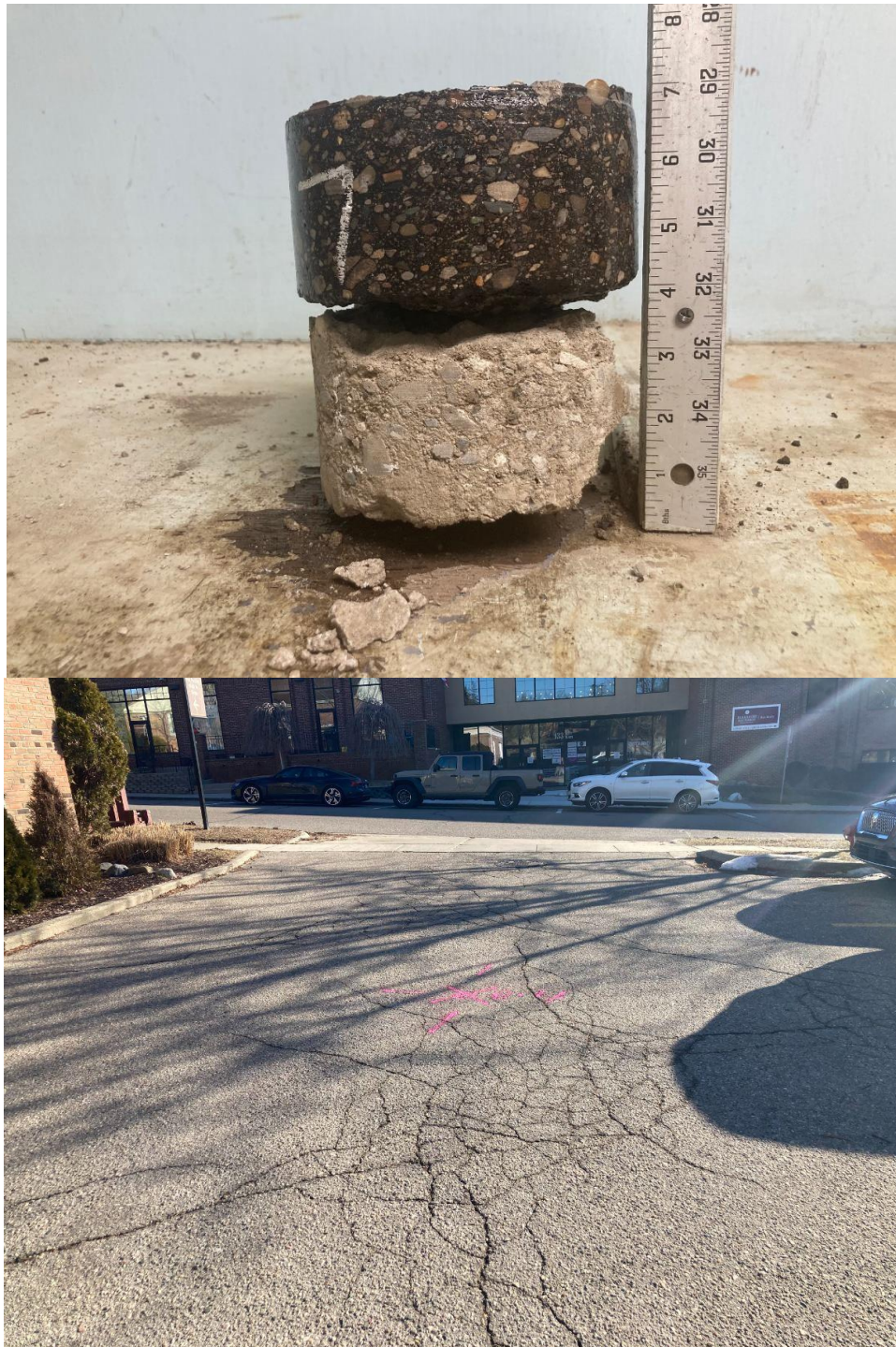
Core Photograph of B-7: Bituminous Concrete = 3-1/4 inches
