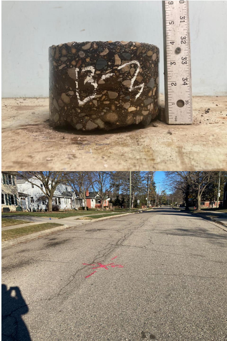
Core Photograph of B-3: Bituminous Concrete = 4 inches
