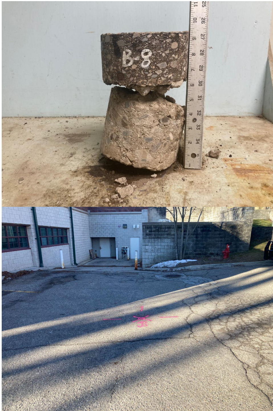
Core Photograph of B-8: Bituminous Concrete = 3-1/4 inches
