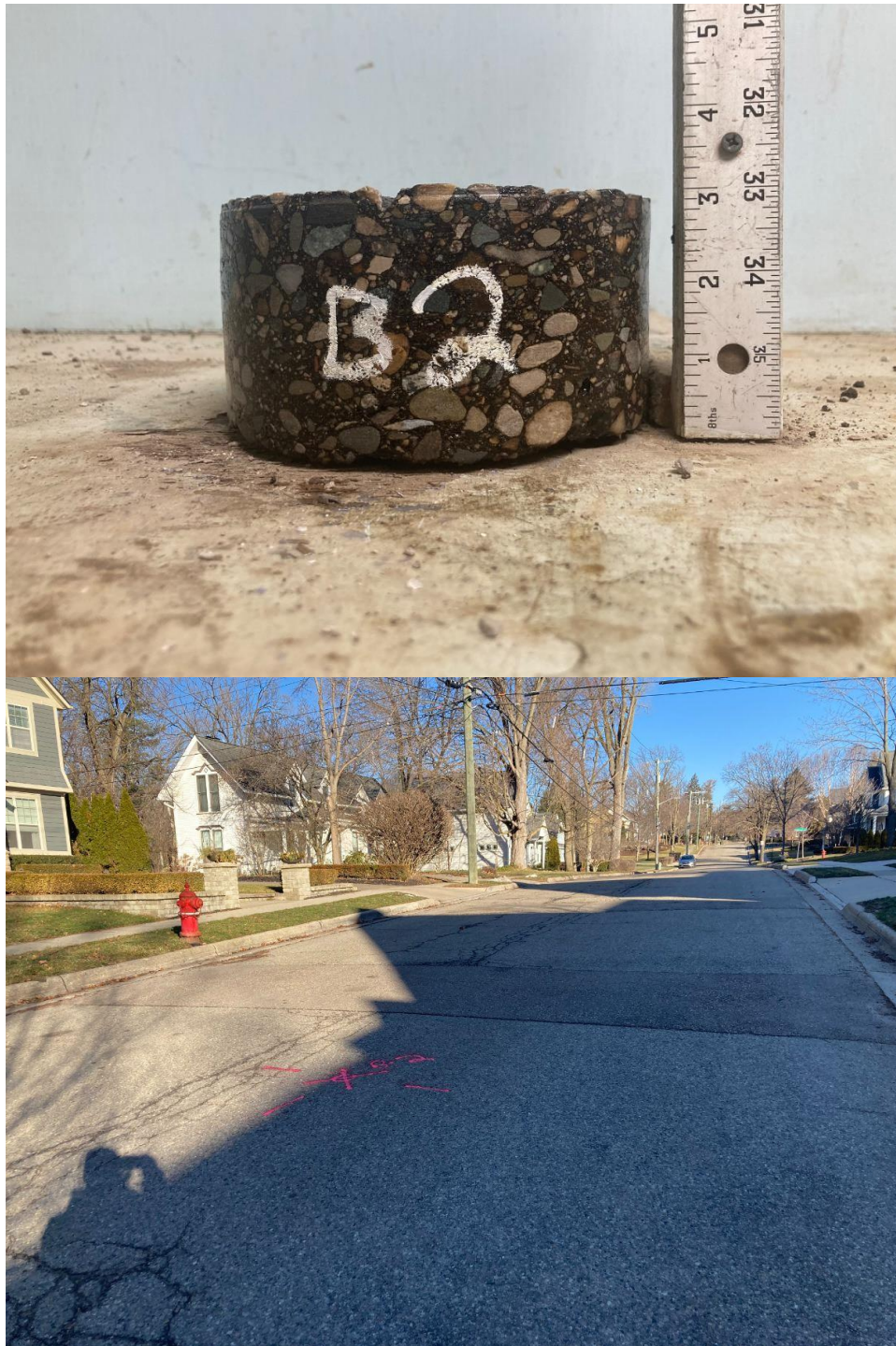
Core Photograph of B-2: Bituminous Concrete = 3 inches
