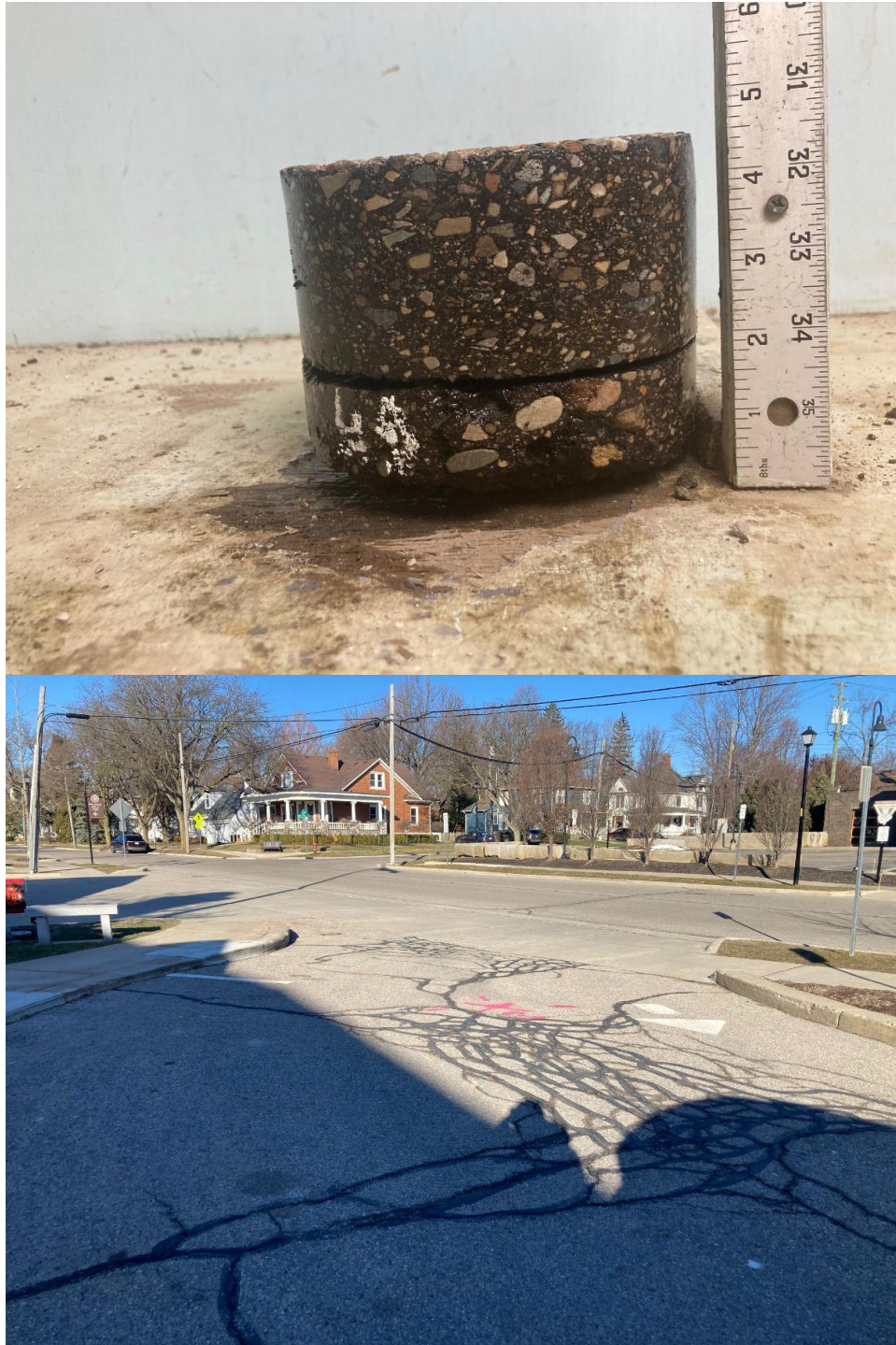
Core Photograph of B-5: Bituminous Concrete = 4-1/2 inches
