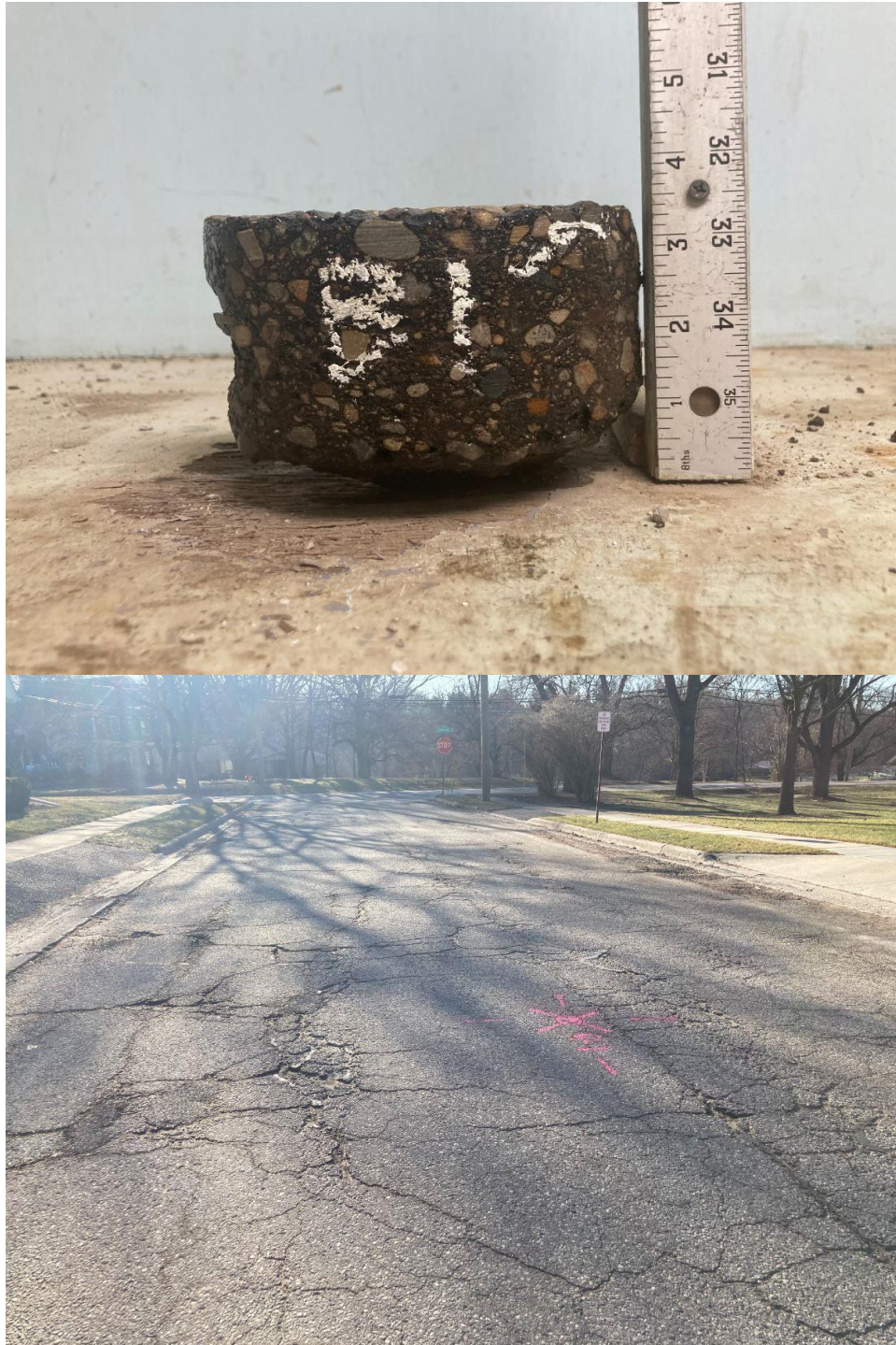
Core Photograph of B-1: Bituminous Concrete = 3-1/2 inches
